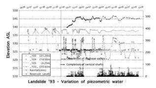
Fig. 8: Piezometric measurements of group II103-II105
