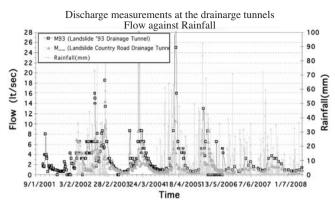
Fig. 16: Discharge measurements at the drainage tunnels in the areas of 1993 Landslide, and Country Road Landslide in relation to the rainfall.
