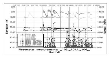
Fig. 13: Piezometric Measurements of Group  $\Gamma$ 102,  $\Gamma$ 104A,  $\Gamma$ 108A and  $\Gamma$ 106a & b.
