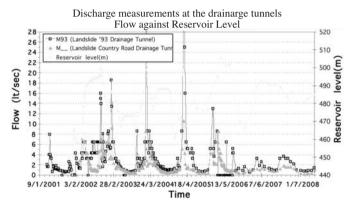
Fig. 17: Discharge measurements at the drainage tunnels in the areas of 1993 Landslide, and Country Road Landslide in relation to the reservoir level.
