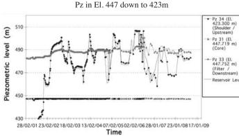
Evolution of piezometric level with time in Section IX-
