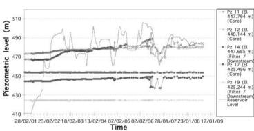
Evolution of piezometric level with time in Section VI Pz in El. 448 down to 425m
