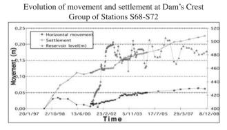
Fig. 5: Cumulative mean displacements and settlement in the dam's Crest.
