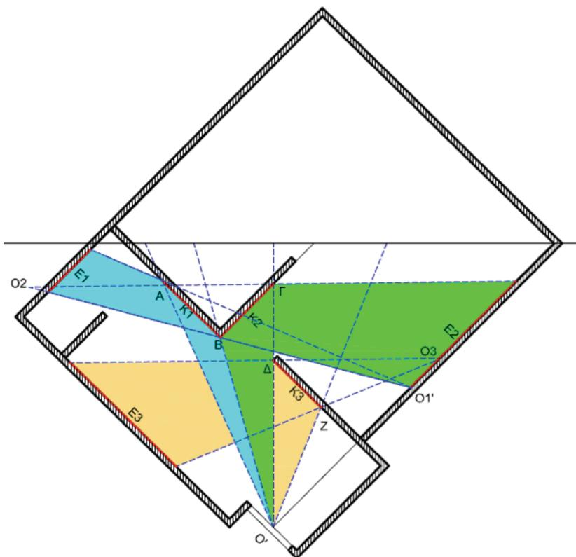
Fig.3 The floor plan of the room, the point of view of the observer and the construction process.
