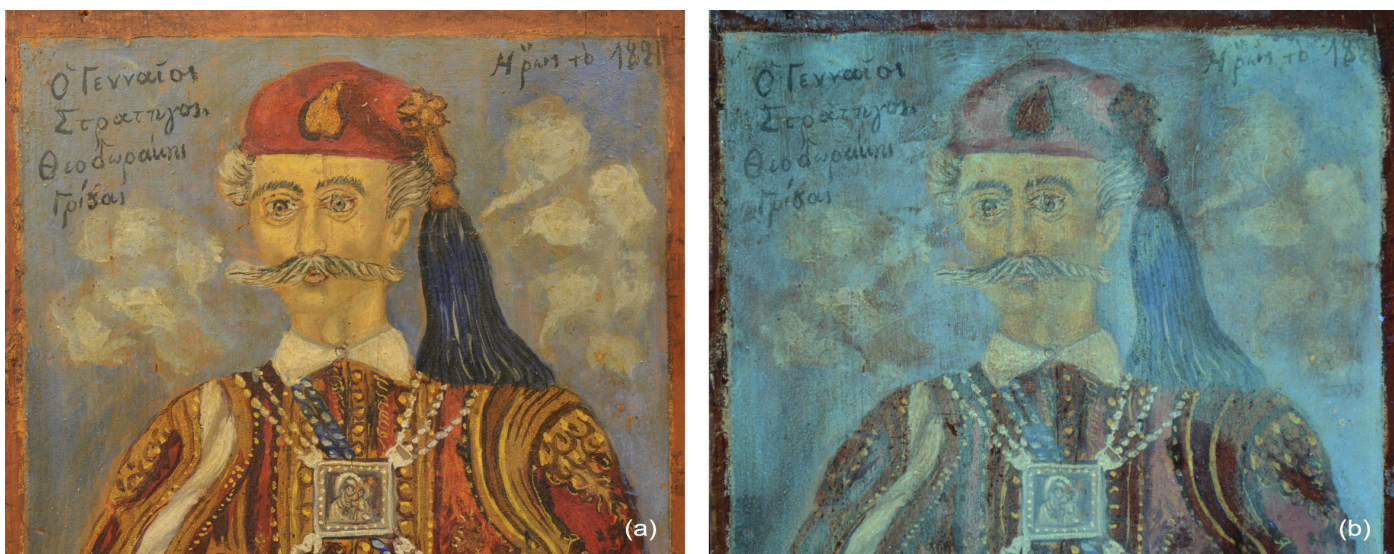
Figure 2: Theophilos, The brave general Theodorakis Grivas, after 1929, tempera on wood, 62.7x23.5cm, Athens, Museum of Modern Greek Culture (no.2808) – detail. (a) visible light photography, (b) ultraviolet induced visible fluorescence photography. (Alexopoulou A. and Kaminari A., 2016)
