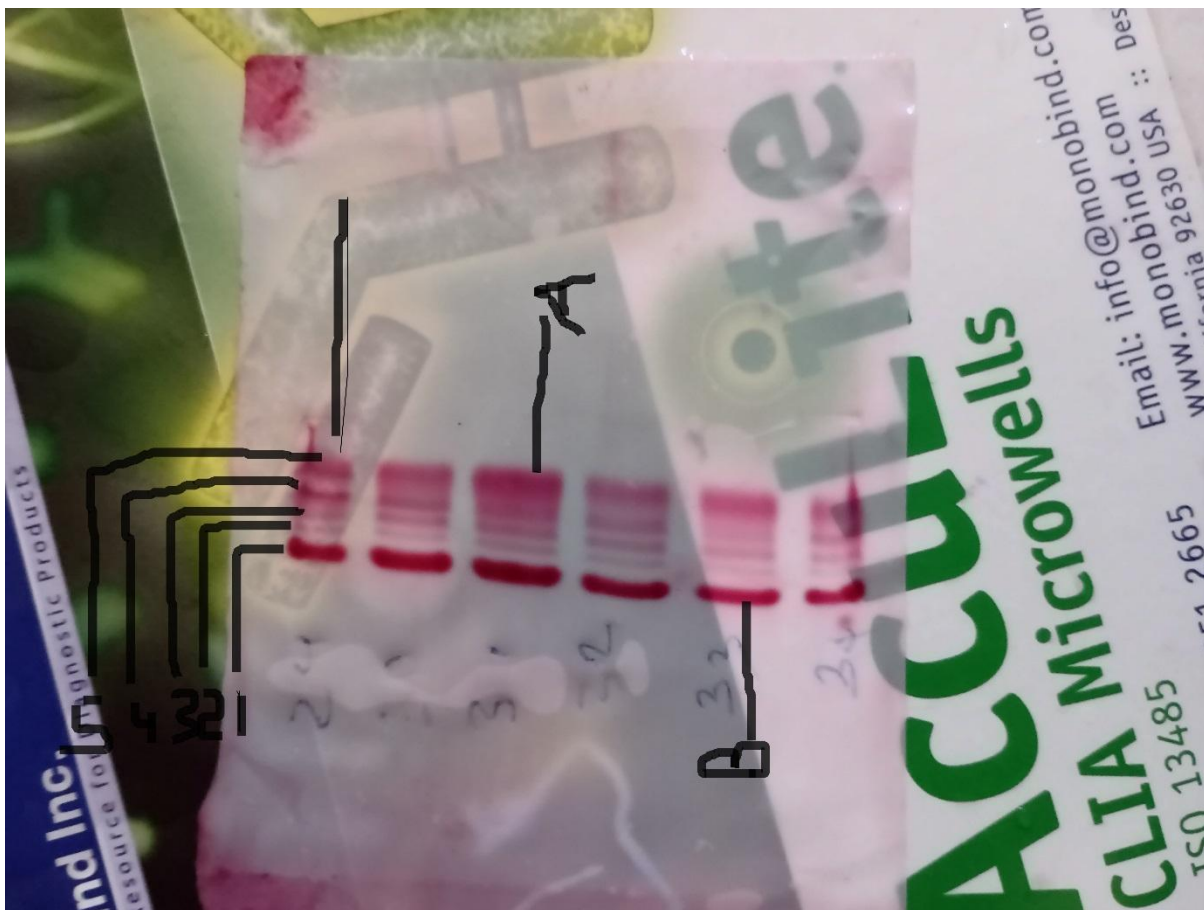
FIGURE 1. Electrophoregram showing different protein bands, albumin, \alpha_1 , \alpha_2 , \beta and \gamma globulins.
