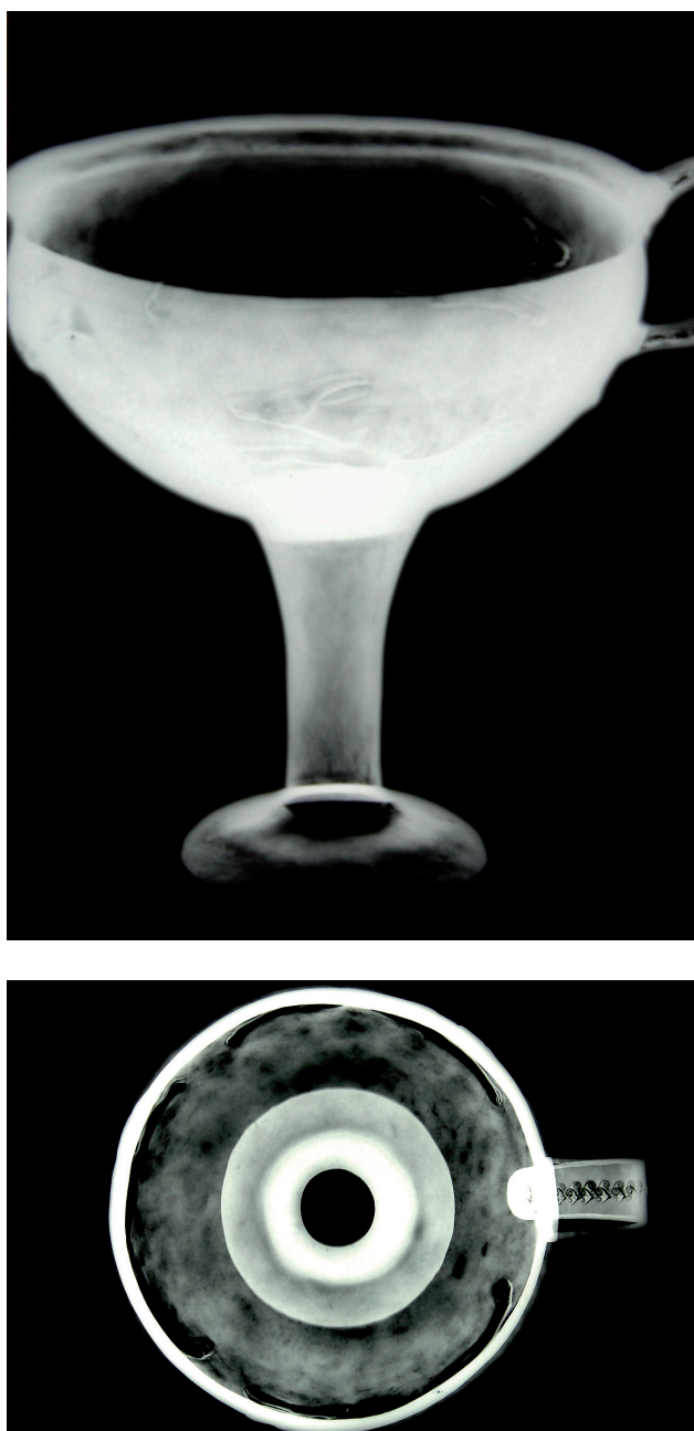
Fig. 2a-b. X-ray image of the kylix, showing a) the marks left by the tool used for the hammering process; b) the attachment areas between body, foot and base; c) the way the foot was formed from a coiled sheet of gold hammered into shape (the joining of its edges is visible); d) the circular centre mark on the base of the body. Athens, Benaki Museum, inv. no. 2108.
