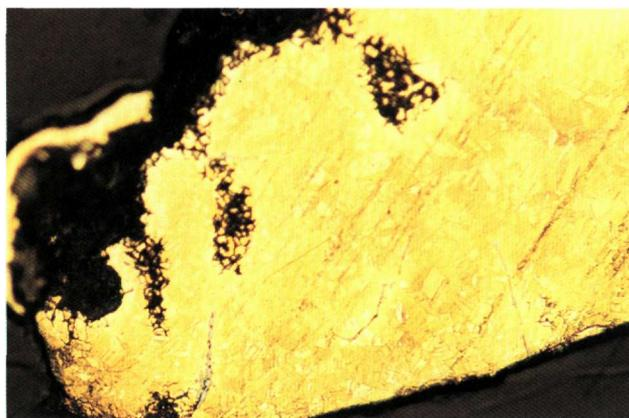
Figs 5-6. Cross section details of the body sample under bright field unpolarized illumination and polarized illumination. Etch:  $\text{FeCl}_3$  x 200: a. Homogenous structure, b. Slip lines, grain deformation, annealing twins emerging on grain boundary facets, c. Hair line cracks especially around the surface of the samples, d. Intergranular corrosion (few areas), e. No inclusions.
