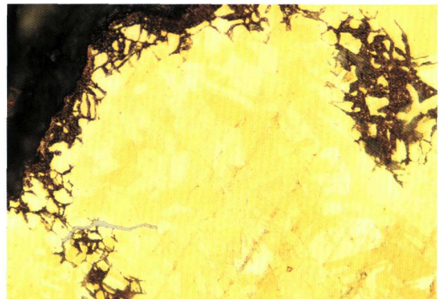
Fig. 12. The light blue elongated inclusions in cross section. Etch: \text{FeCl}_3 x 1000.
