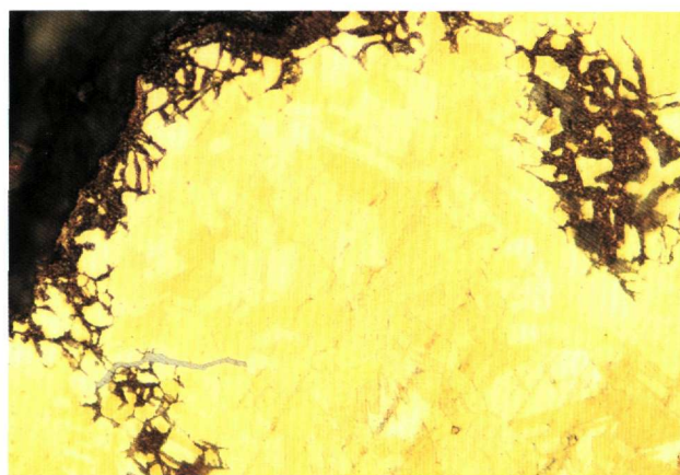
Fig. 12. The light blue elongated inclusions in cross section. Etch: \text{FeCl}_3 x 1000.
