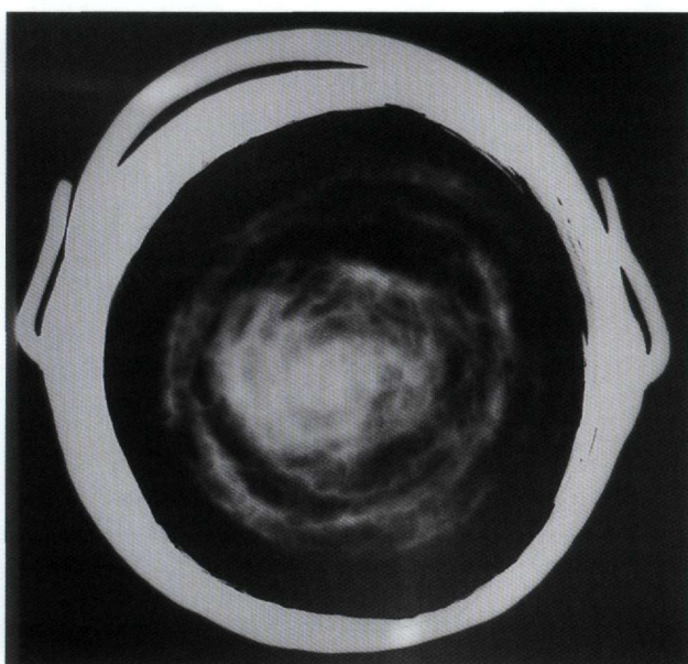
Fig. 4. X-ray image of the interior, showing tool marks produced by hammering.
