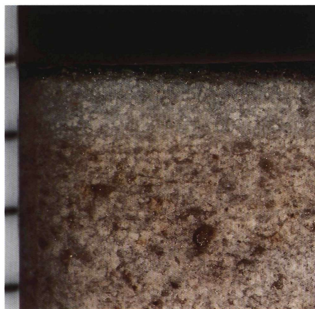
Figs 4, 5. Thin section 40x and cross section 30x. The slip layer is more dense and fine-grained than the ceramic body. Crystal size in the slip does not exceed 40 \mu\text{m} whereas silica crystals in the ceramic body can reach up to 45 \mu\text{m} .
