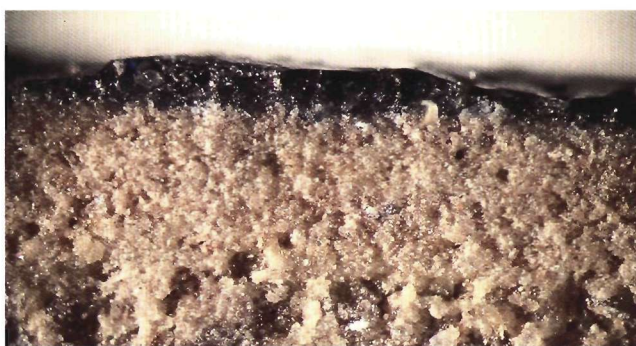
Fig. 2. Tile no. 92, cross section, 60x. Note the 150-200 \mu\text{m} -thick transparent glaze layer.
