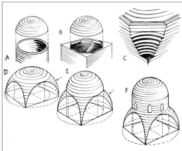
Figure 2. Dome development: Diagrams (after D. YARWOOD, *The Architecture of Europe: The Ancient Classical and Byzantine World, 3000 BC-AD 1453*, London: B. T. Batsford Ltd, 1992, fig. 175). A: Dome over cylinder B: Dome over square with squinches across corners to make an octagon C: Squinch D: Pendentives integral with dome E: Pendentives independent of dome F: Dome raised on a drum.
