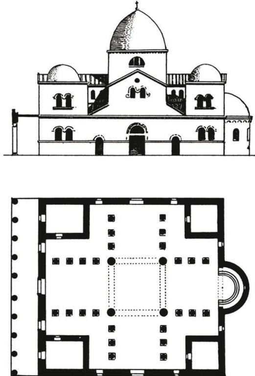
Figure 12. Cross-in-square regular church type: Church of the Prophets, Martyrs & Apostles, Gerasa, elevation and plan, AD 464-5 (E. Baldwin SMITH, *The Dome: A Study in the History of Ideas*. Princeton, NJ: Princeton University Press, 1971, figs 175 & 177).
