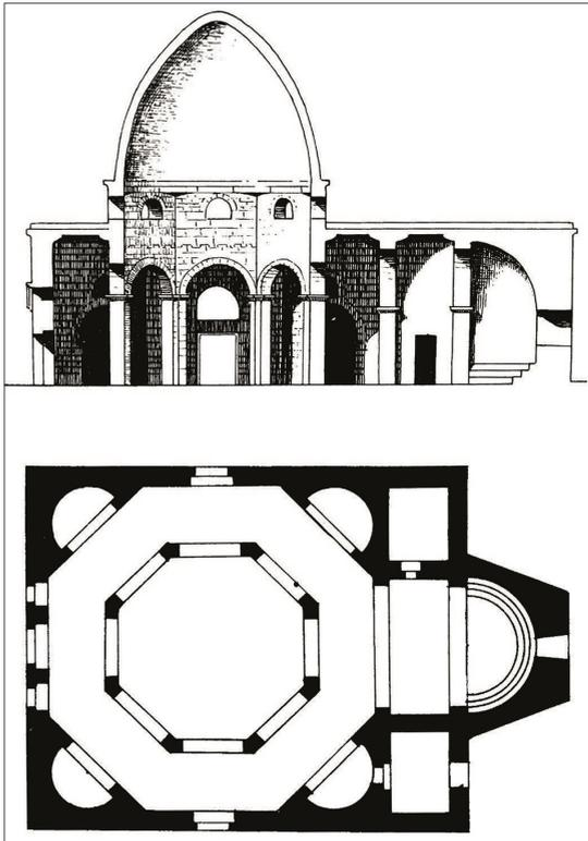
Figure 4. Near East conical dome: St. George Martyrium, Zorah, section & plan, AD 515 (E. Baldwin SMITH, *The Dome: A Study in the History of Ideas*. Princeton, NJ: Princeton University Press, 1971, figs. 50 & 51).
