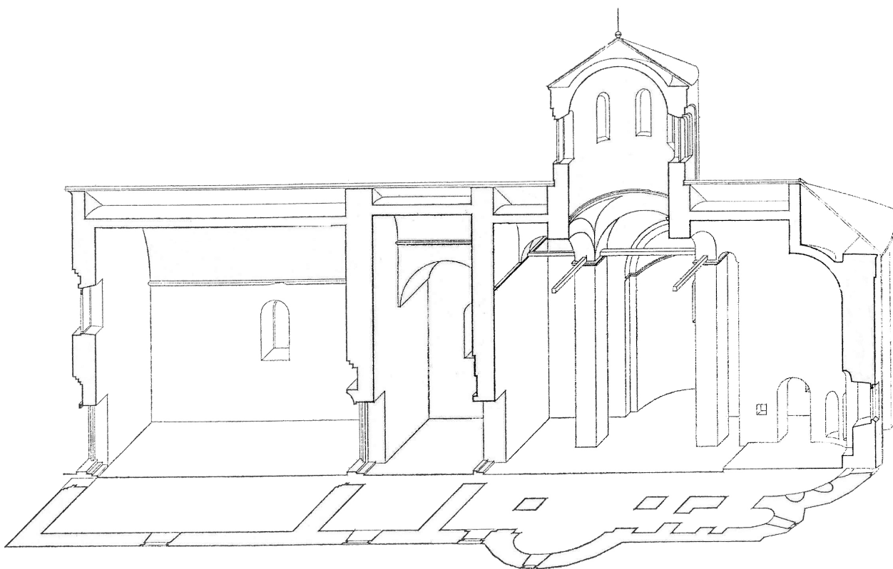
Fig. 4. Serbia, monastery of Papraća, church of the Annunciation. Axonometric section.
