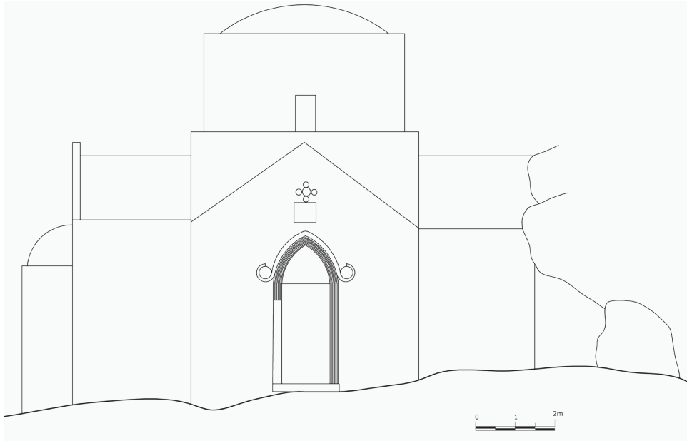
Fig. 18. Schematic drawing of the north façade of the church of Panagia in Prinós (Rethymnon), showing the location of bacini.
