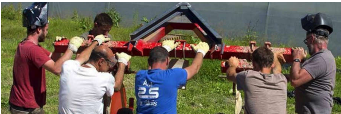
Picture 2: Construction of the quick hitch triangle
