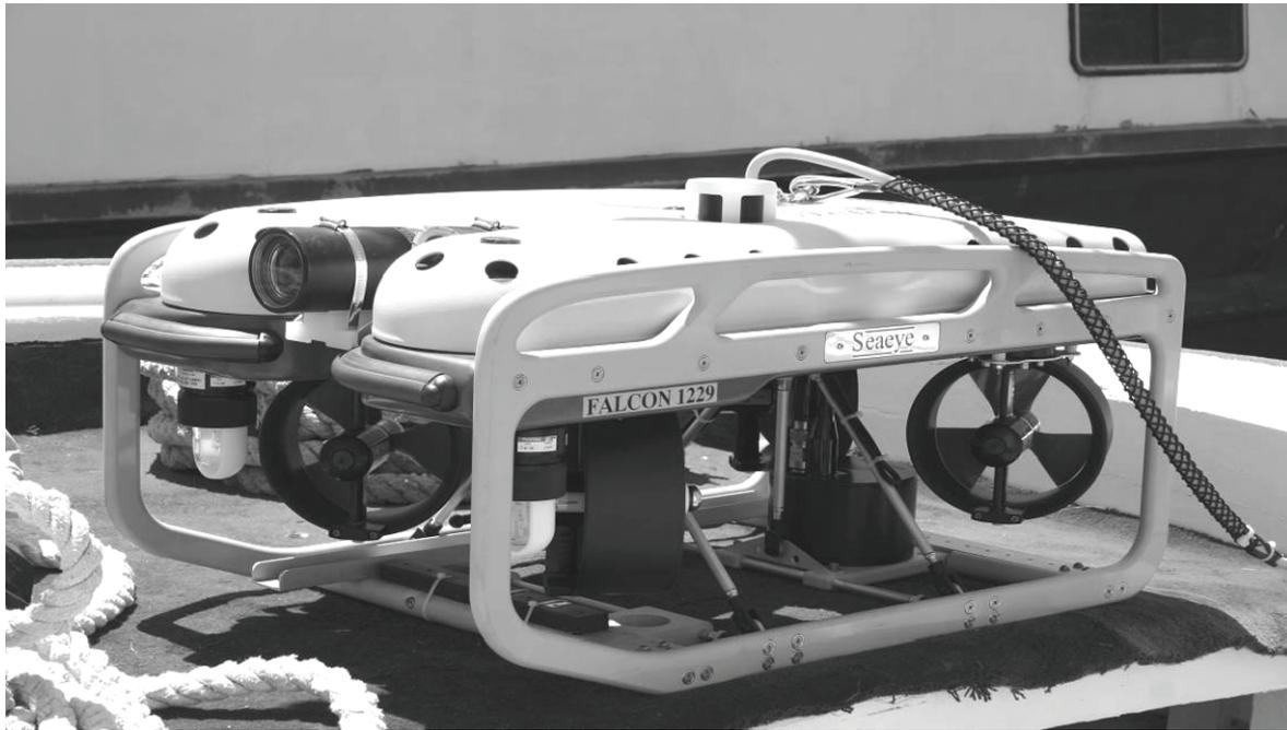
Fig. 3 Remote Operated Vehicle used in 2004 survey.
