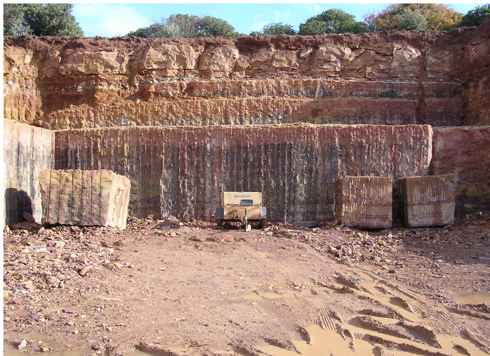
Fig. 2. Quarrying front showing the four commercial types of the Thymianá Stone.
