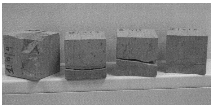
Fig. 4. “Hemískliri”; Splitting and separation across anisotropy planes in specimens having undergone freeze - thaw cycles.
