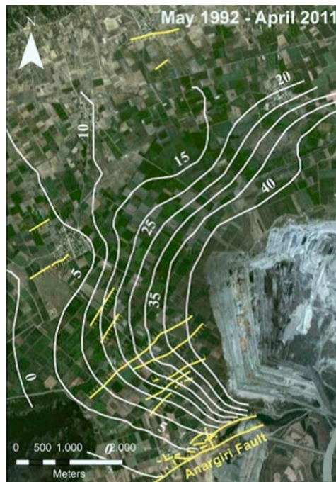
Figure 4 - Drawdown contour lines map drawn by subtracting the piezometric surfaces of May 1992 (Dimitrakopoulos, 2001) from the ones of April 2011 (Aggelitsa, 2012; Loupasakis et al. , 2014).
