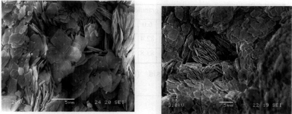
Figure 7 - SEM images of the platy hydromagnesite/magnesite mineral assemblages of the bulk sample Can-2. Even magnesite has platy texture, making almost impossible its distinction from hydromagnesite by SEM-EDS analysis. In the right image, late stage magnesite-hydromagnesite crystals are filling a pore
