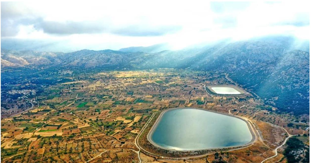
**Fig.S10** SE part of Lasithi Plateau from above (Spring 2020). The figure illustrates the two artificial reservoirs for irrigation purposes, as Aposelemis project's compensation measure. Photo taken by Spyros Lianakis and displayed with his permission.
