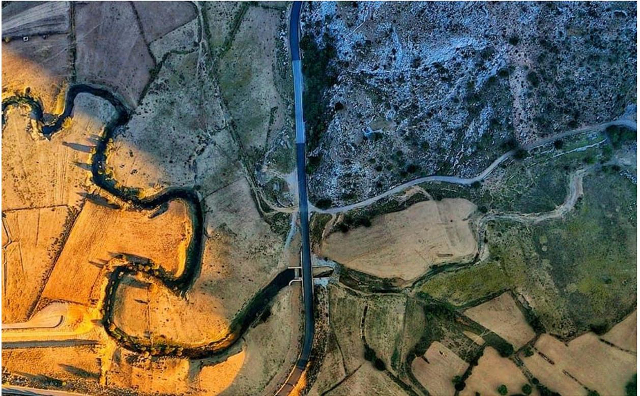
**Fig.S9** NW part of Lasithi Plateau from above (Spring 2020). The figure illustrates Chavgas stream. Sinkhole isolation work at the road's bridge puts a stop to the streamflow. At the middle right Chonos sinkhole can be seen. At the bottom left, part of the main trench of the project is illustrated. Photo taken by Spyros Lianakis and displayed with his permission.
