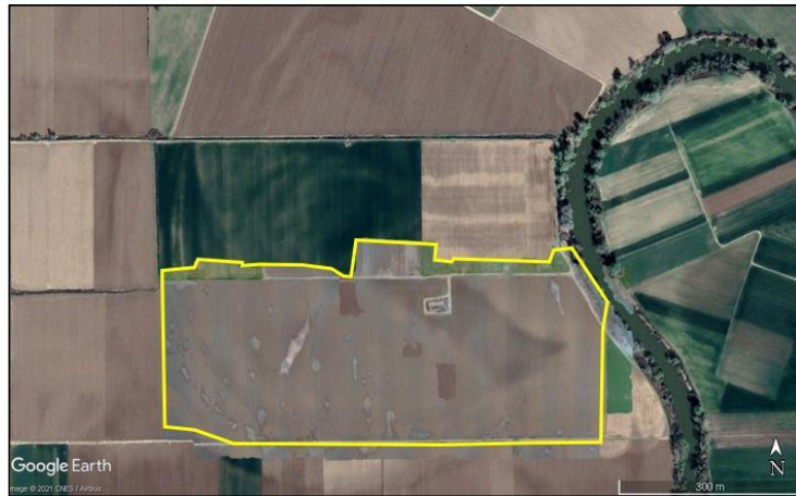
Fig. 14: A detailed UAV composite orthophoto (yellow border) overprinted onto a satellite image, clearly shows that the distribution of individual liquefaction features (gray spots) coincides with an abandoned and filled bend of Pinios river. The current riverbed is visible at the right part of the map.
