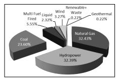
Figure 1 - Share of the sources of Turkey's installed capacity for power generation (from EÜAS, 2011)
