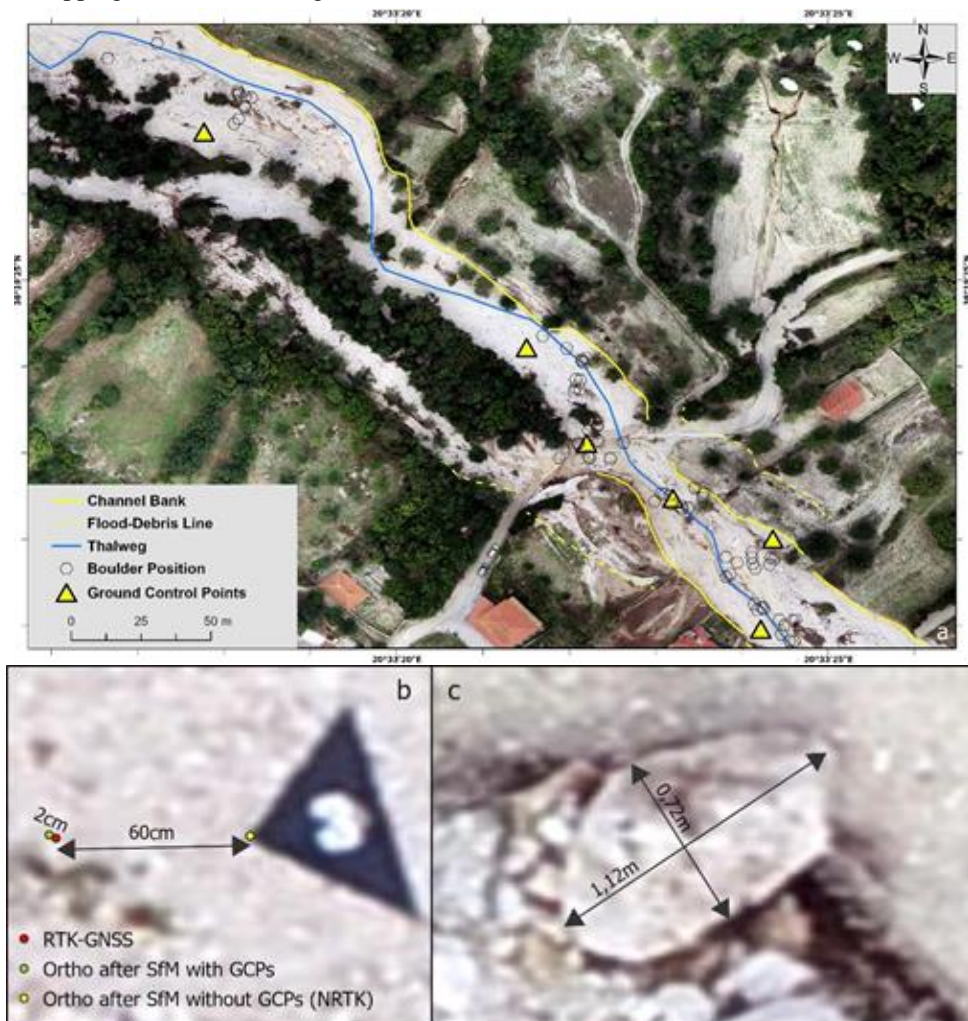
Figure 1. (a) Interpretation of the experiment river segment (see legend for symbol meanings). (b) Checking the accuracy of the final ortho-photo-mosaic with the precise coordinates of the GCP. (c) Accurately measuring the a and b axes of a boulder.
