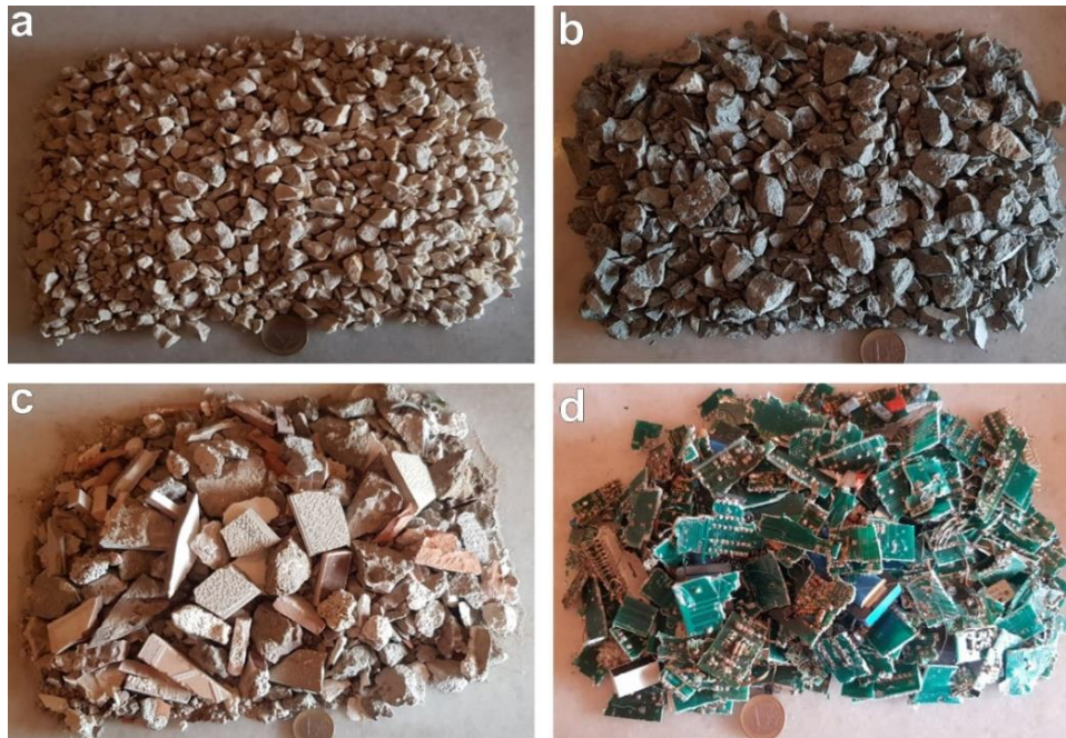
Figure 2. Representative photos of aggregate components showing: (a) Limestone; (b) Basalt; (c) construction wastes; (d) E-wastes.
