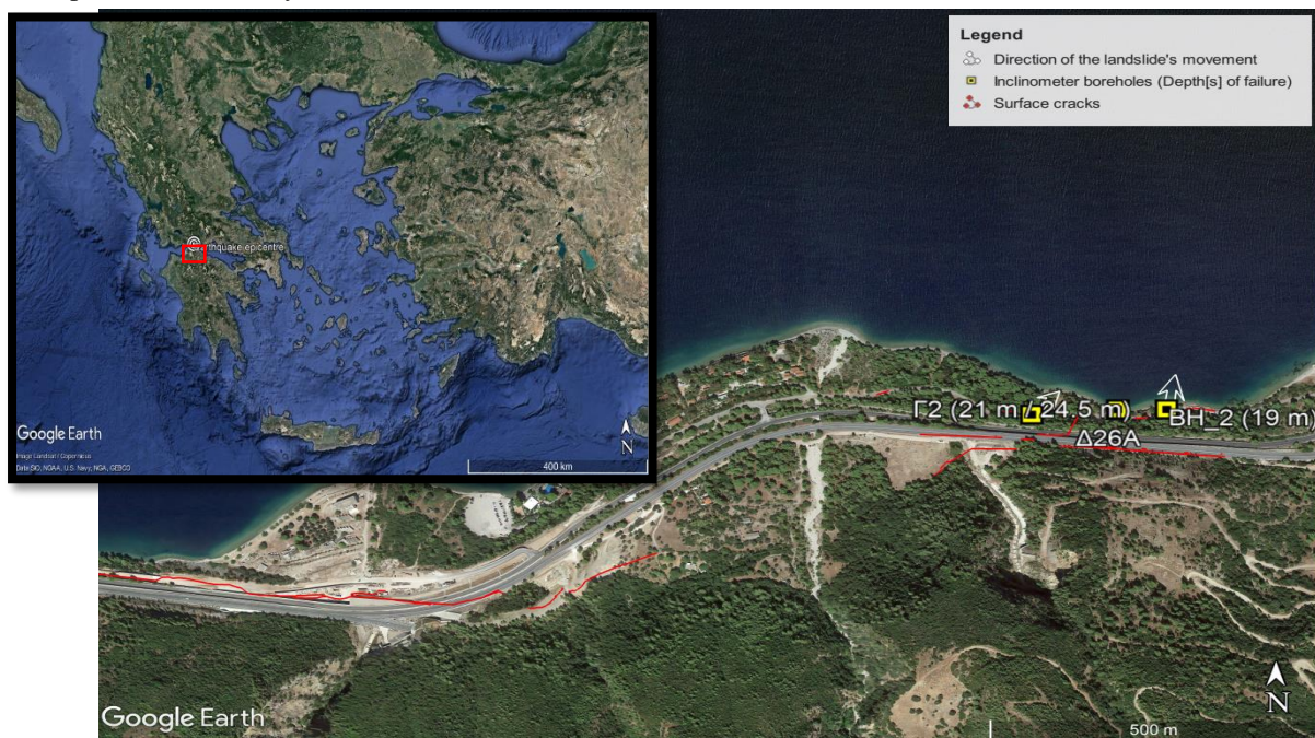
Figure 1: The wider area of the Panagopoula landslide with its movement characteristics and crack development after the seismic event of 17.02.2021.
