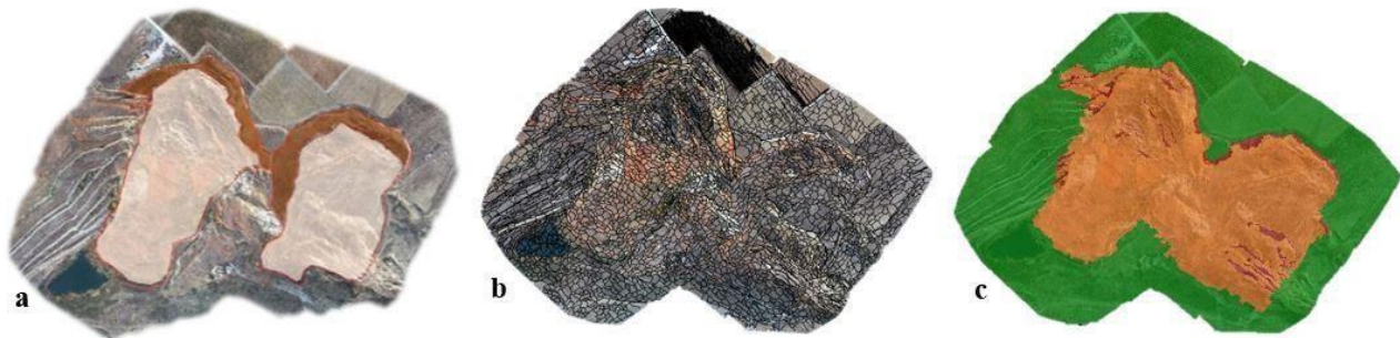
Figure 2. a) Orthophoto overlaid by the reference data, b) segmentation result and c) the final classification after refinement of the rule-based method (green: non-affected, light brown: depletion, dark brown: scarp).
