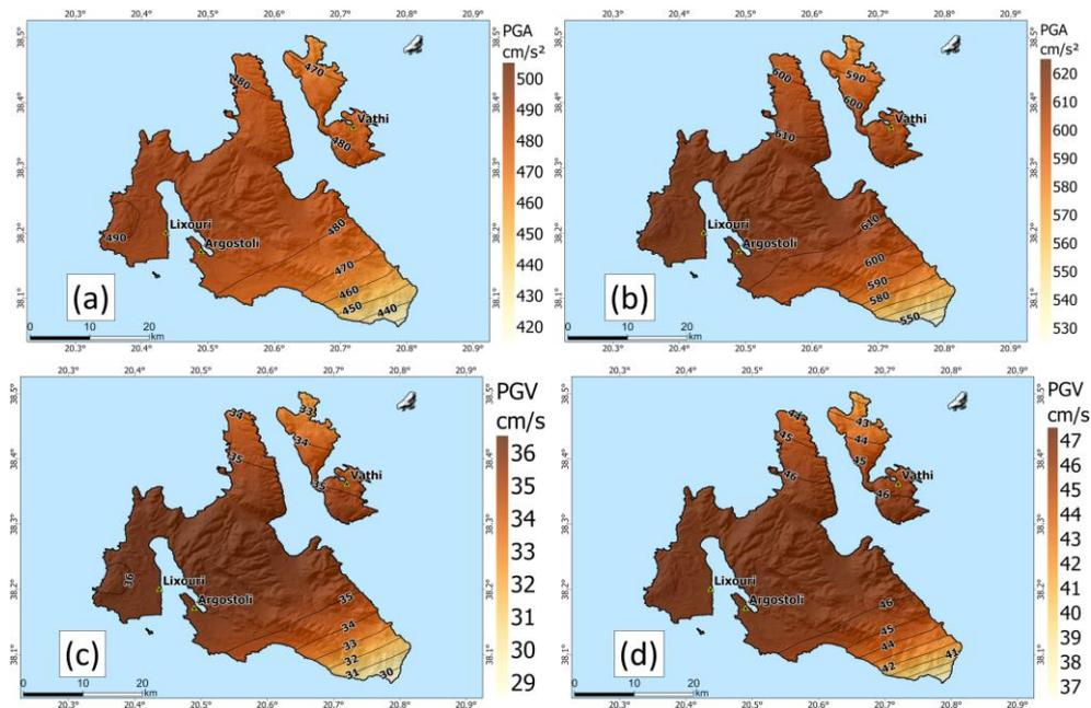
**Figure 3. Maps showing the spatial distribution of PGA (a, b) and PGV (c, d) for RPs of 475 years (left) and 950 years (right).**
