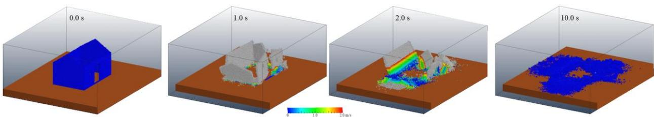
**Figure 4. Snapshots of a discrete element model of building #3 from OBB under the load of a 1 Hz cycloidal pulse parallel to the longitudinal side of the structure (time of frames given on top). The color bar indicates the instantaneous velocity of elements; values above 2.0 m/s are in gray.**
