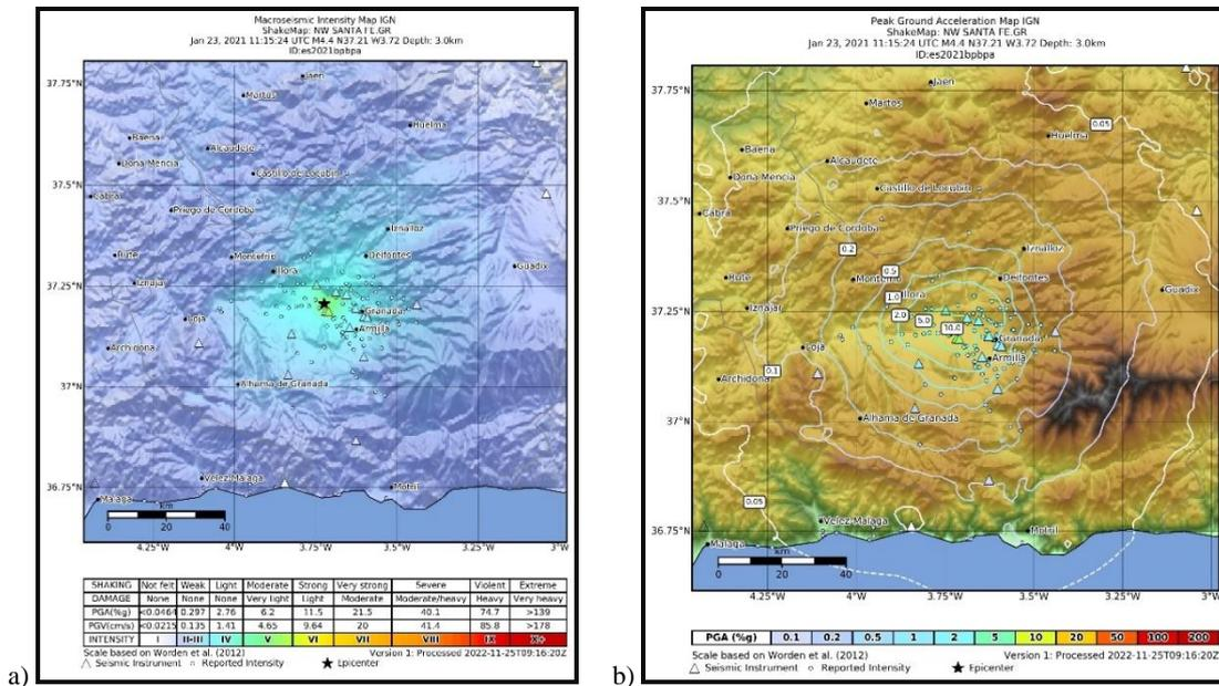
**Figure 2. Examples of Shakemaps for 23/01/2021 Granada earthquake in terms of intensity and in terms of Peak Ground acceleration. (Source: Instituto Geográfico Nacional)**
