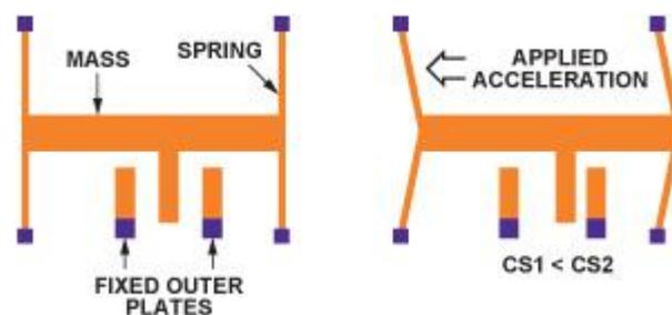
**Figure 3. MEMS accelerometer (capacitive microsensor) [Figure obtained from O'Reilly *et al.*, 2009]**
