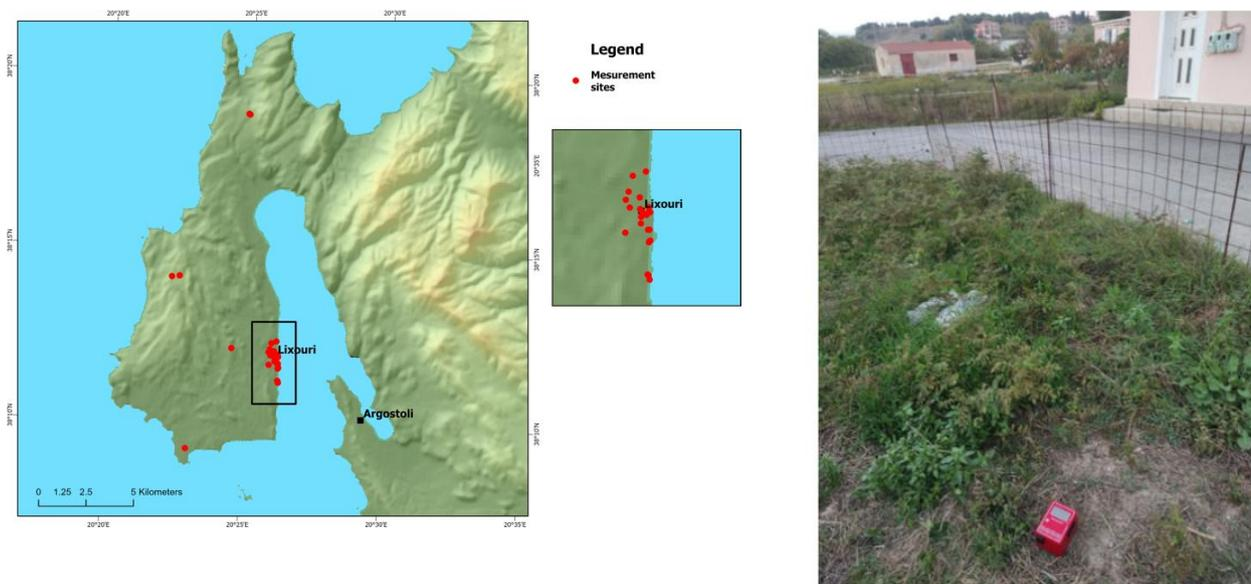
**Figure 1. Left: Map showing spatial distribution of ambient noise measurements, at the instruments sites (red circles). Right: Tromino measurement.**
