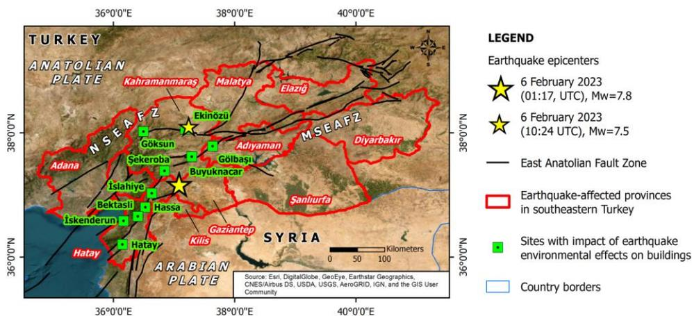
**Figure 1.** The provinces in southeastern Turkey affected by the 6 February 2023 earthquakes due to rupture of the East Anatolian Fault Zone (EAFZ). The sites where the earthquake environmental effects greatly affected the building stock are presented with green symbols and green letters. Red colors in symbols and letters correspond to the affected provinces. MSEAFZ: Main Strand of the EAFZ; NSEAFZ: Northern Strand of the EAFZ.
