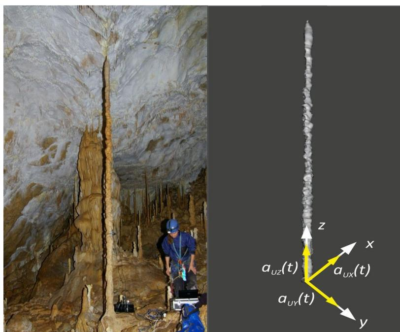
**Figure 2. Photograph of 4.3m stalagmite in Plavecká Priepast cave and system of geometric axes applied in its analysis (X-EW, Y-SN, Z-UP) and its seismic accelerations ( $a_{UX}$ ,  $a_{UY}$ ,  $a_{UZ}$ ).**
