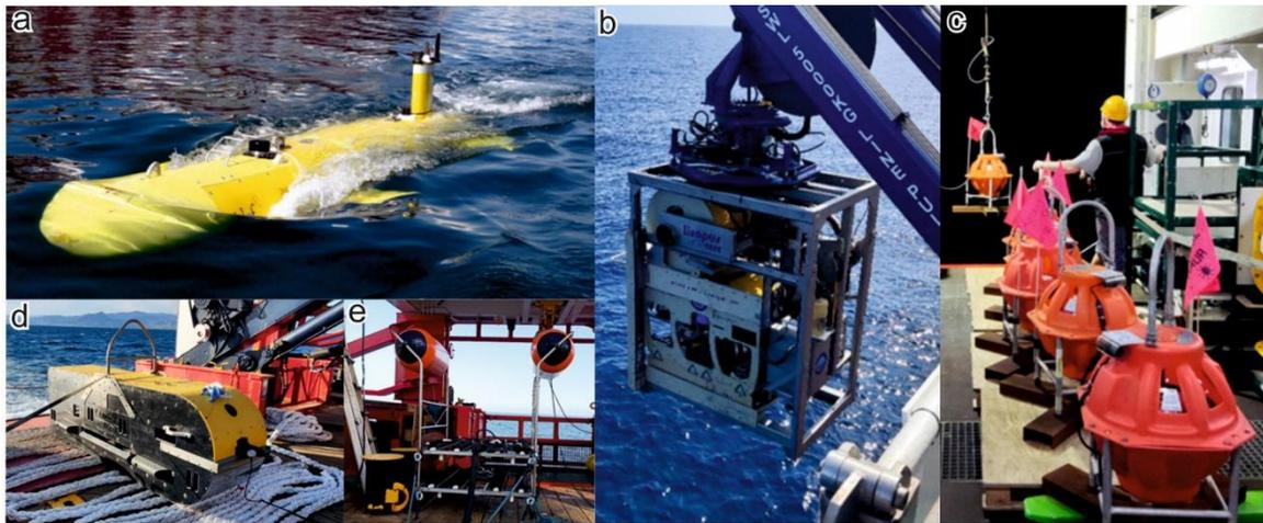
**Figure 2. High-technological equipment used during the STRENGTH cruise. a) Autonomous Underwater Vehicle (AUV) AsterX (Ifremer, France); b) Remotely Operated Vehicles (ROV) Liropus (IEO, Spain); c) Ocean Bottom Seismometers (OBS) (Ifremer, France, and UTM, Spain); d) high-resolution side scan sonar DT-1 Edgetech (UTM, Spain); and e) high-resolution sparker seismic system (UTM, Spain).**
