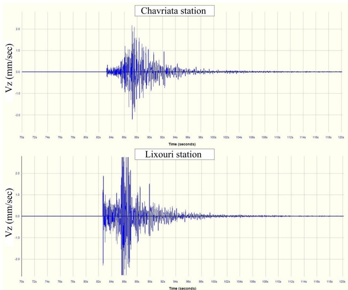
**Figure 2. The vertical component ( $V_z$ ) of the recorded velocity (in mm/sec) of a seismic event on 7 July 2023 of magnitude  $M_w$  3.6 and focal depth 10 km from the station in Chavriata village (top) and the station in Lixouri (bottom)**
