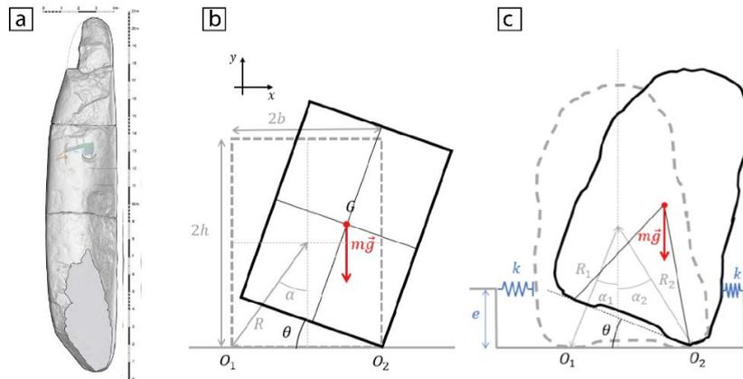
*Figure 2: a) Sketch of the ‘Grand Menhir Brisé’. b) Model 1: rectangular block model (Housner, 1963). c) Model 2: Buried precarious block model adapted from Shi et al. (1996).*
