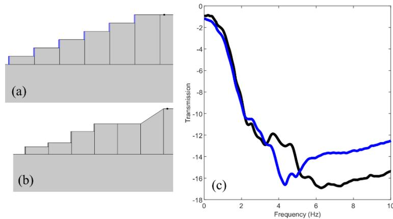
**Figure 3.** The examined terraced slope with concrete walls (a), the relevant non periodic case (b), and the Transmission for each examined case. Case (a) is represented by the black line, and case (b) is represented by the blue line.
