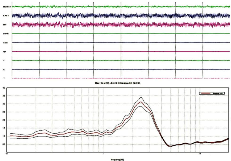
**Figure 3. Ambient noise record at ELTA site in Lixouri (top) and HVSR results processed with Grilla<sup>®</sup> software (bottom).**
