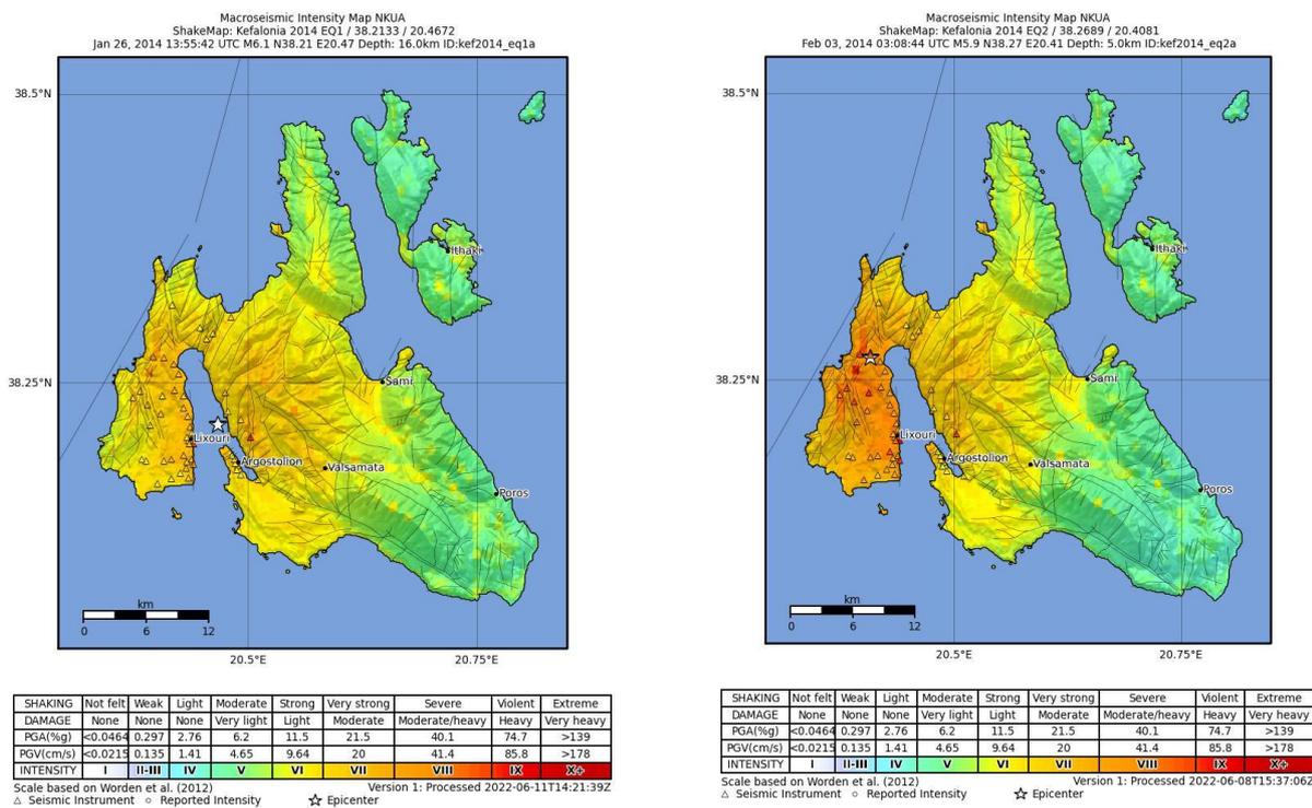
**Figure 1. Example of ShakeMaps from the 2014 Mw6.1 and Mw5.9 earthquakes in Kefalonia, Greece. Images from the National and Kapodistrian University of Athens.**
