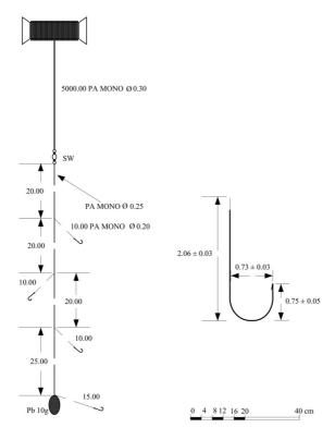
Fig. 2: Technical plan of fishing lines used in experiments.
