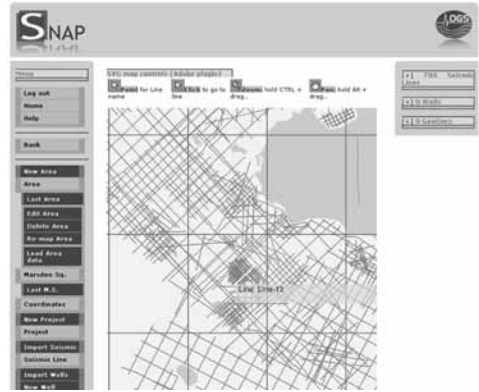
Fig. 3: Within an SVG map objects remain such. They are isolated and react independently. Here in a quite cluttered area it is easy to identify a seismic line. Clicking on it the system sends the user to a page listing the data available.
