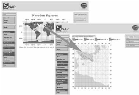
Fig. 4: Using Marsden Squares it is possible to precompute maps to be cached server-side in order to reduce the time required for compilation and rendering of a map created from scratch.
