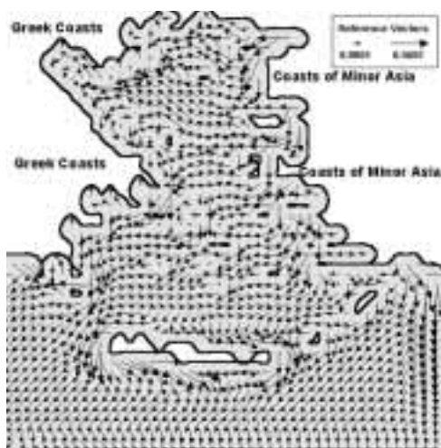
Fig. 4a: Current velocities of the upper layer under the Etesians for 3 days (ref vectors in m/s).
