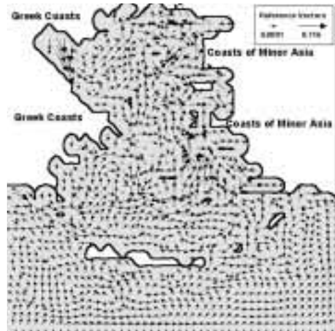
Fig. 8b: Current velocities of the lower layer under the Etesians for 6 days (ref vectors in m/s).
