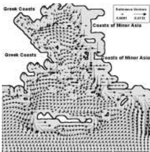
Fig. 4b: Current velocities of the upper layer under the Etesians for 6 days (ref vectors in m/s).
