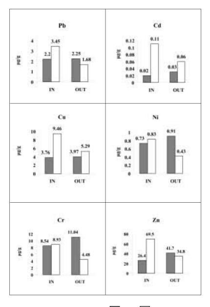
Fig. 7: Metal content of particulate matter ( $\mu g/g$ )
