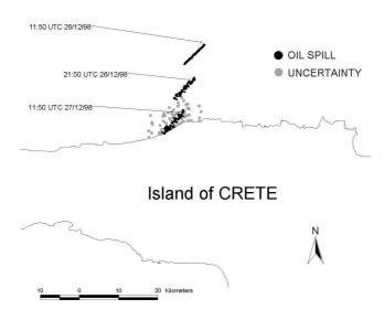
*Fig. 5:* Simulated oil spill scenario using GNOME software.
