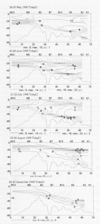
Fig. 4: The temperature transects in the Strait of Istanbul and its south and north approaches.
