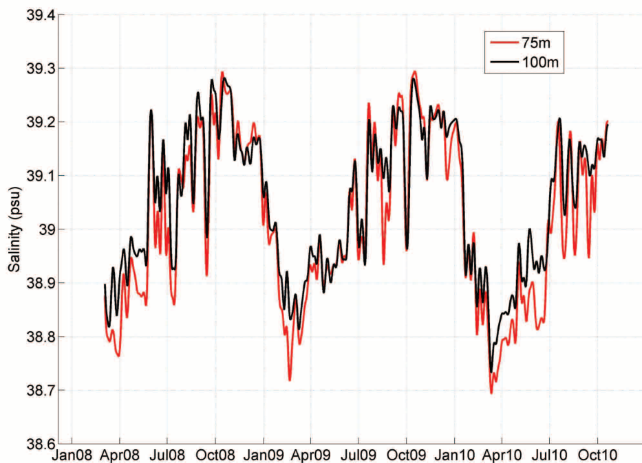
Fig. 6: Athos station. Time series of salinity at 75 and 100 m depth (January 2008–October 2010).
