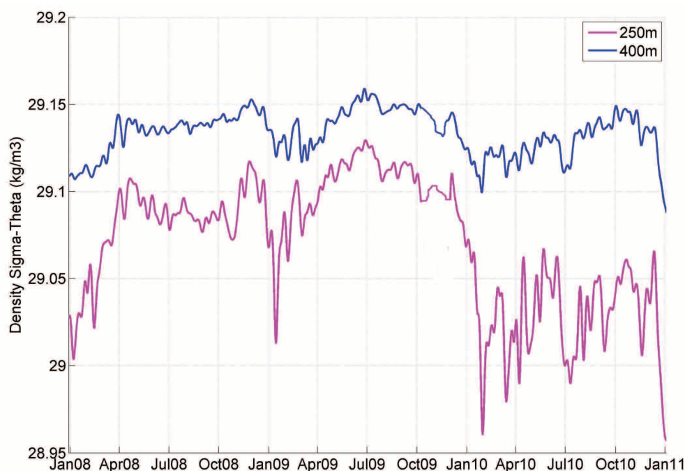
Fig. 20: Pylos station. Time series of potential density ( \sigma_\theta ) at 250 and 400 m depth (January 2008–January 2011).
