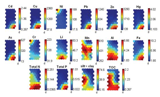
*Fig. 3:* Component planes of the SOM for the chemical variables (input variables or components): trace and major elements, TOC% and fine grain fraction ( $<0.63 \mu m$ ). Hexagons in a certain position in each plane correspond to the same map unit in Figure 2. The value of the component in the weight vector (distance) of each unit of the map is represented by the colours in the scale bar (right side of each component plane).
