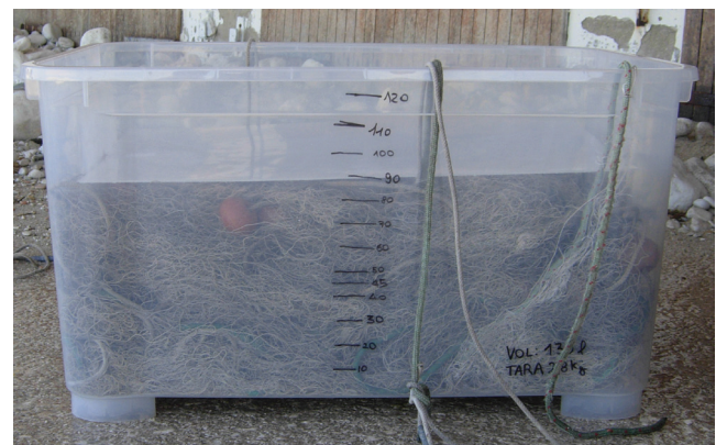
Fig. 2: Graduated container used for the evaluation of the net volume.
