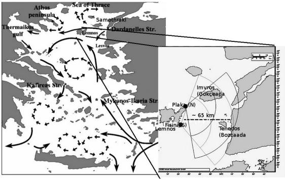
*Fig. 1:* The study Area. Presentation of the surface circulation and the radar coverage of each site, as is provided by H. Messtechnick. The horizontal distance of the radar coverage area is  $\sim 65$ km and the elevations of the two main islands that are inside the area of radar coverage are 12m for Tenedos and 673m for Imvros.
