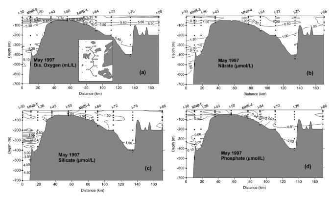
Fig. 7: Dissolved Oxygen and nutrient transects from the LW area towards the north Lemnos area during May 1997.
