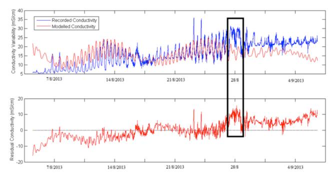
*Fig. 4*: a) Upper panel: Water conductivity in Ismarida Lake, as recorded by the auto-recording hydrographic station (blue line) and water conductivity reconstruction model, based on harmonic analysis results (red line); b) Lower panel: Residual (no-tidal) fluctuation of water conductivity variability in Ismarida Lake. Rectangle represents the period of the fish mortality event.
