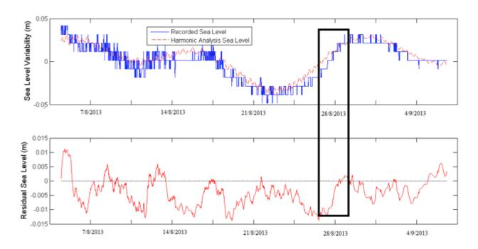
*Fig. 3*: a) Upper panel: Water level variability in Ismarida Lake, as recorded by the auto-recording hydrographic station (blue line) and water level reconstruction model, based on harmonic analysis results (red line); b) Lower panel: Residual (non-tidal) fluctuation of sea level variability in Ismarida Lake. Rectangle represents the period of the fish mortality event.
