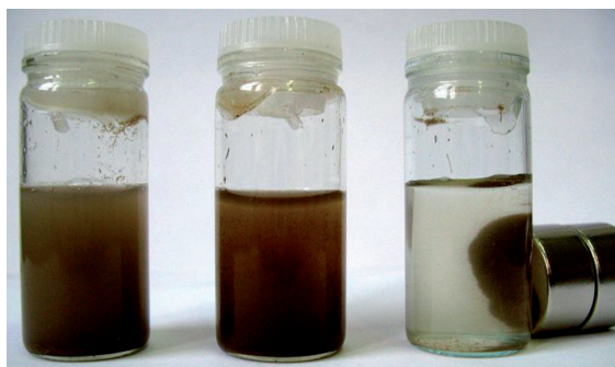
Fig. 6: Appearance of original Posidonia biomass suspension (left), suspension of biomass after magnetic modification (middle) and demonstration of magnetic separation of magnetically modified biomass (right).
