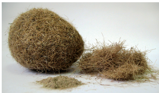
Fig. 2: Posidonia oceanica fibres ball, separated fibres and fine biomass particles obtained by milling.
