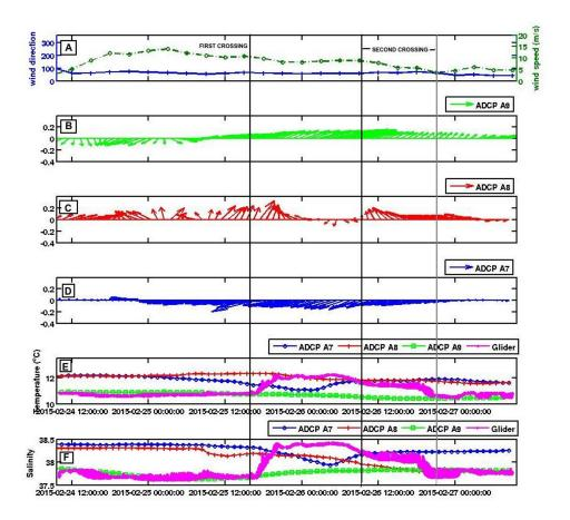
Fig. 2: A) Wind from ALADIN/HR model, B) ADCP A9 station, depth-averaged current measurements, C) ADCP A8 station, depth-averaged current measurements, E) Temperature plot of the ADCPs stations bottom measurements and the glider data, F) Salinity plot of the ADCPs stations bottom measurements and the glider data. The black vertical lines are depicting the two times when the glider was crossing the IF. The gray line refers to the time that the glider finished the second crossing. Hours are GMT.
