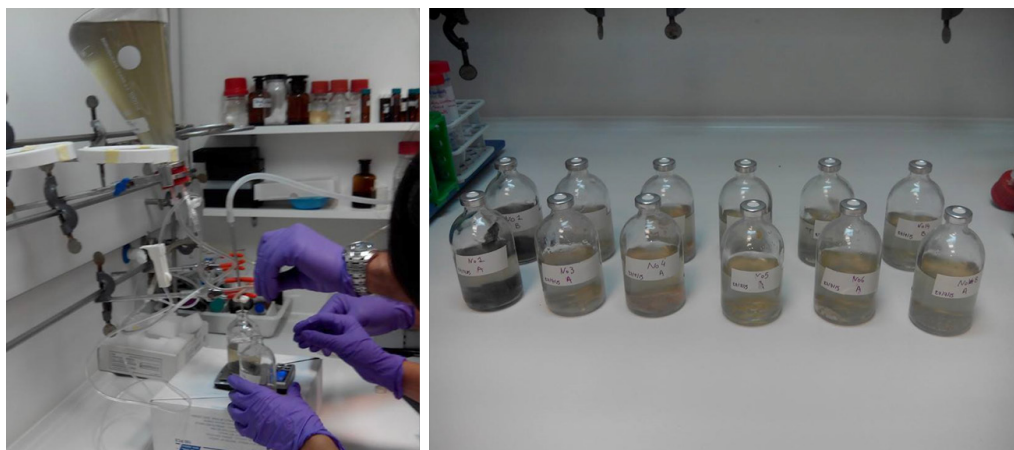
Fig. S2: Transfer of the culture medium into serum bottles under anaerobic conditions and preparation of multiple cultures for the investigation of methane production.
