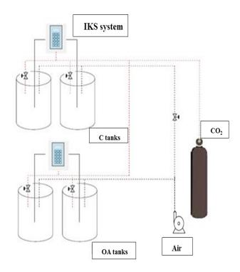
*Fig. 2:* Design of the experimental set-up demonstrating the two tanks for each pH treatment (OA and C), the IKS system monitoring the CO<sub>2</sub> gas supply and the air pump providing air to the systems.
