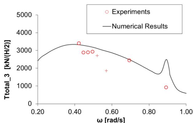
Fig. 27: Mooring tensions comparisons on the 3<sup>rd</sup> OWC.
