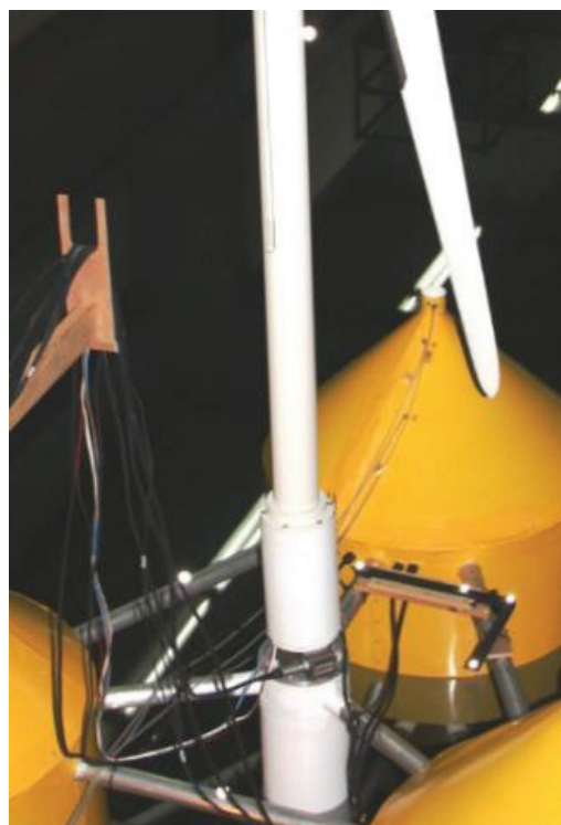
Fig. 11: Accelerometers and optical targets for motion recording.
