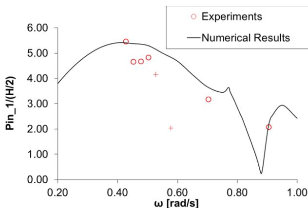
Fig. 24: Air pressure inside the 1<sup>st</sup> OWC of the platform. Comparisons with experimental results.
