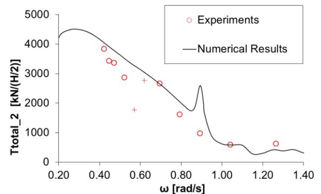
Fig. 18: Mooring tensions comparisons on the 2<sup>nd</sup> OWC.
