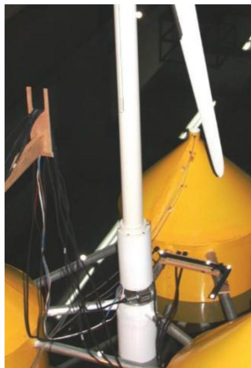
**Fig. 11:** Accelerometers and optical targets for motion recording.
