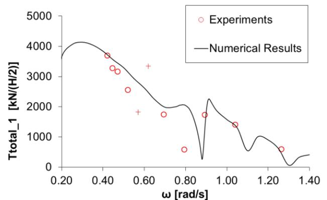
Fig. 17: Mooring tensions comparisons on the 1<sup>st</sup> OWC.
