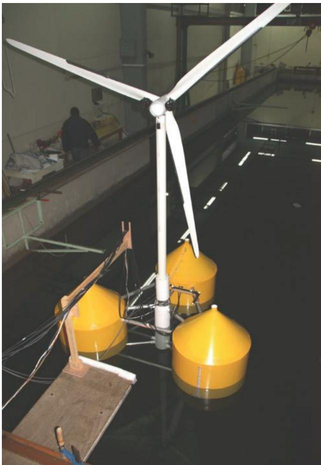
**Fig. 8:** Scale down model of the platform (scale 1:40).
