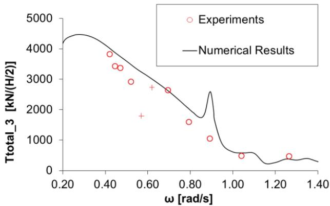
Fig. 19: Mooring tensions comparisons on the 3<sup>rd</sup> OWC.
