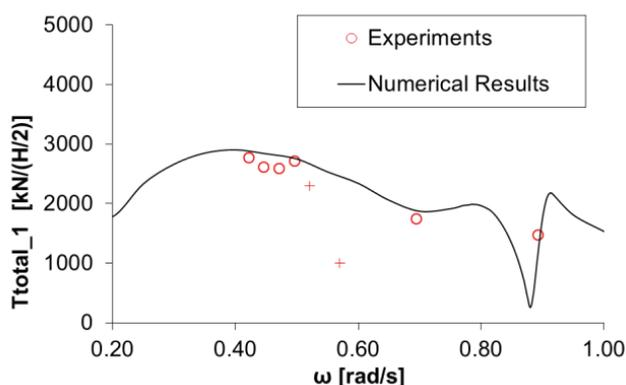
Fig. 25: Mooring tensions comparisons on the 1<sup>st</sup> OWC.
