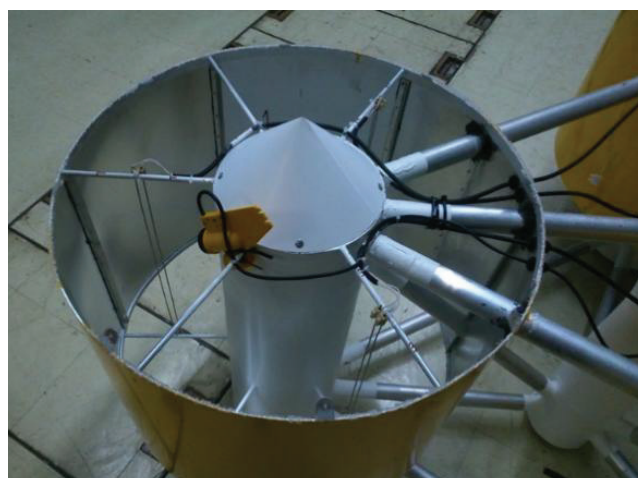
Fig. 10: Wave probes inside the OWC air chamber.
