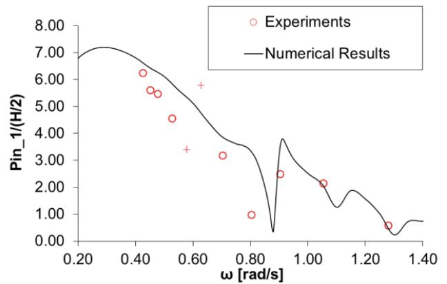
Fig. 16: Air pressure inside the 1<sup>st</sup> OWC of the platform. Comparisons with experimental results.
