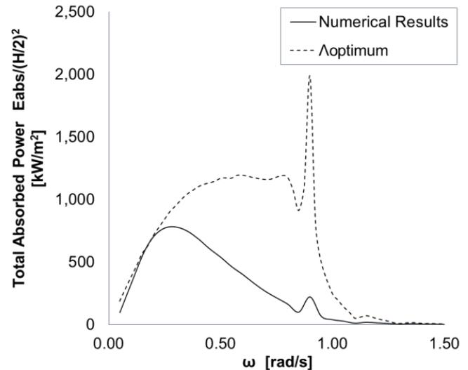
Fig. 22: Total absorbed wave power by the platform for  $\lambda = 0.1$  kN.sec/m<sup>5</sup> and  $\Lambda_{opt}$  coefficients.
