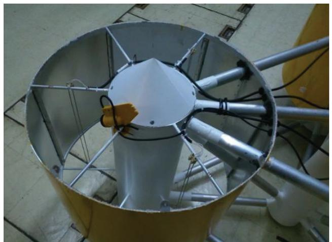
**Fig. 10:** Wave probes inside the OWC air chamber.
