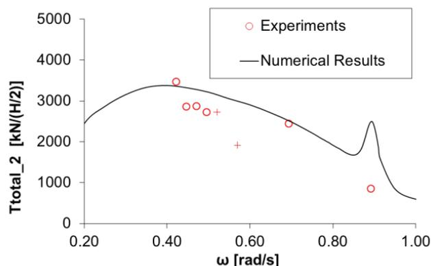
Fig. 26: Mooring tensions comparisons on the 2<sup>nd</sup> OWC.
