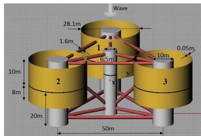
**Fig. 5:** Side view of the buoyant components.
