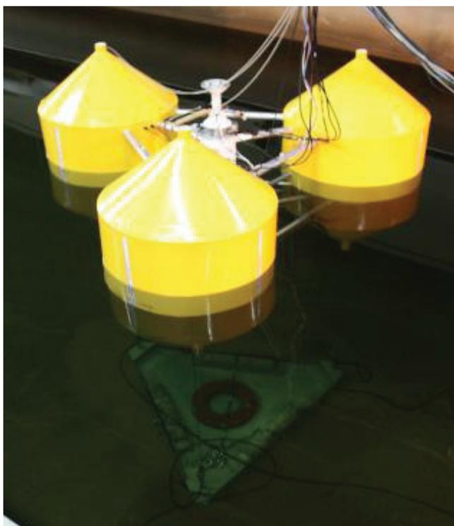
Fig. 12: Base for the TLP mooring system.
