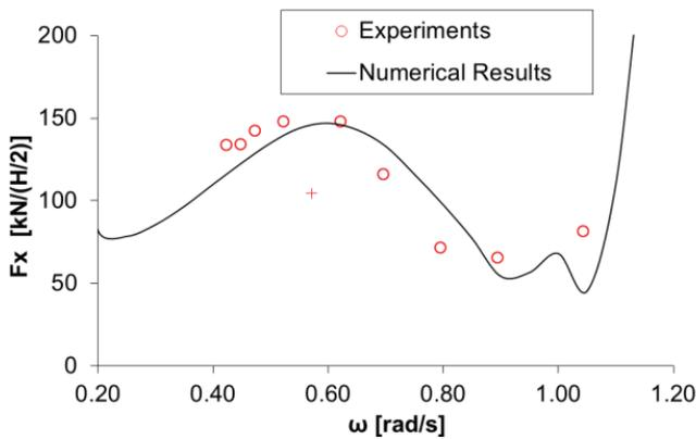
Fig. 20: Comparisons of shear forces at WT base.
