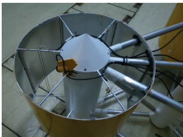
Fig. 10: Wave probes inside the OWC air chamber.
