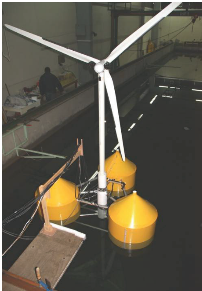
Fig. 8: Scale down model of the platform (scale 1:40).
