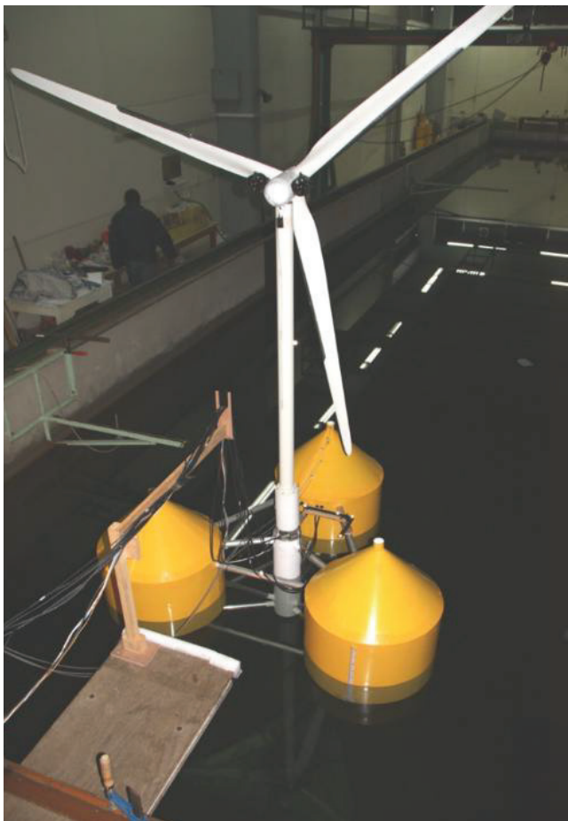
Fig. 8: Scale down model of the platform (scale 1:40).
