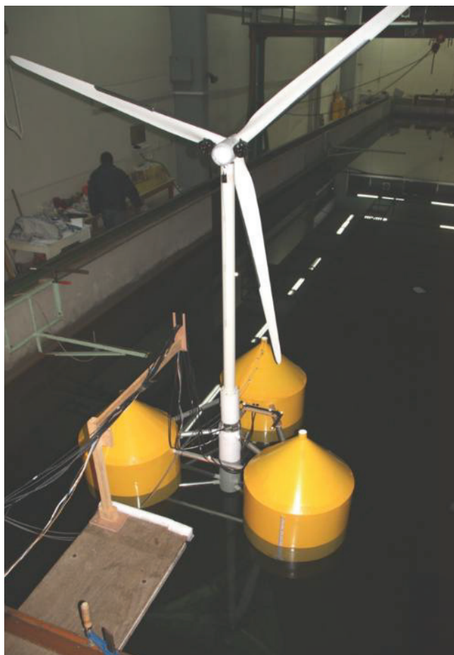
Fig. 8: Scale down model of the platform (scale 1:40).
