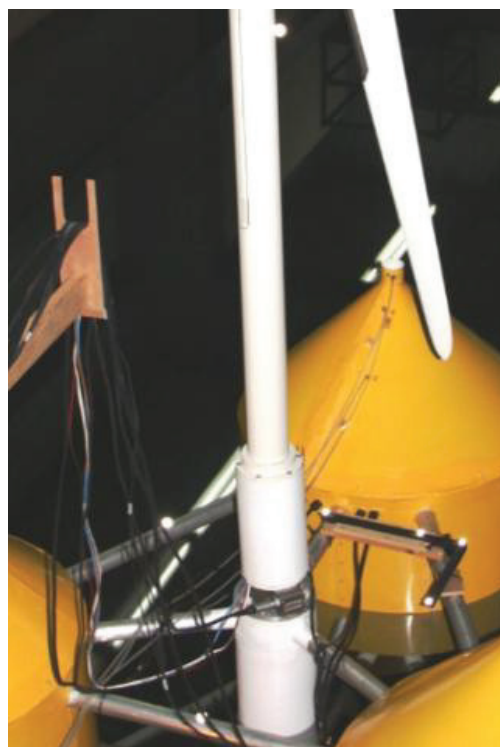
Fig. 11: Accelerometers and optical targets for motion recording.
