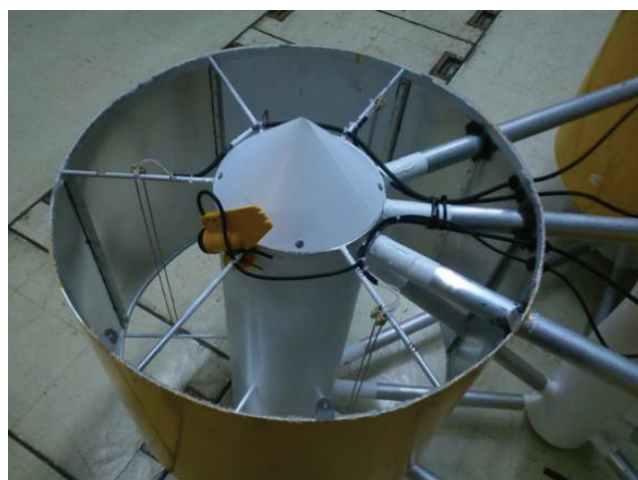
Fig. 10: Wave probes inside the OWC air chamber.
