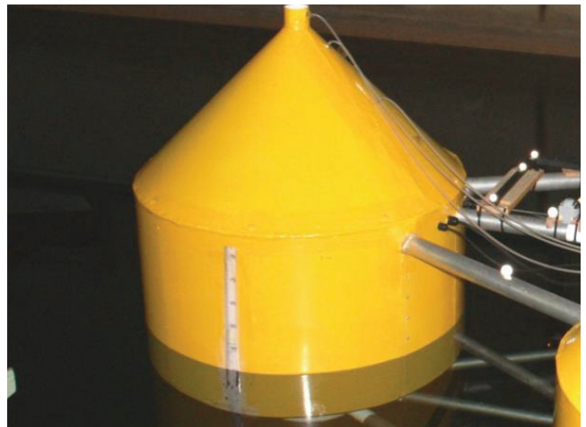
Fig. 9: Three pressure transducers for the pressure inside the front cylinder of the OWC device.
