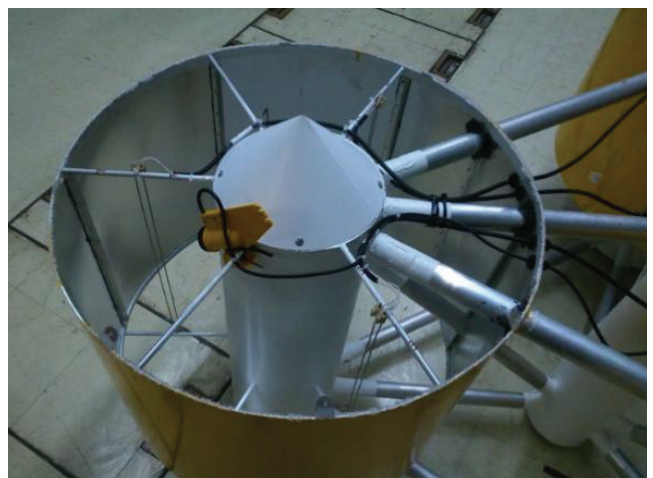
Fig. 10: Wave probes inside the OWC air chamber.
