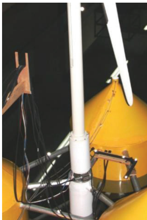
Fig. 11: Accelerometers and optical targets for motion recording.
