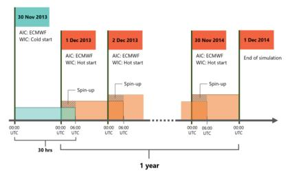
*Fig. 4:* Long-term simulation timeline (Varlas, 2017). Each simulation is initialized at 00:00 UTC and lasts 30 hours starting on 30 November 2013 and ending on 1 December 2014. The crosshatched area represents the spin-up time (00:00-06:00 UTC) of each simulation. The atmospheric initial conditions (AIC) are based on ECMWF analyses while for wave initial conditions (WIC) "cold start" was applied for the 1st day and "hot start" for the rest of the days.
