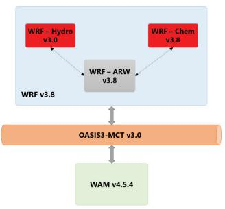
*Fig. 1:* The components of CHAOS (Varlas, 2017; Varlas *et al.*, 2018). WRF-Hydro and WRF-Chem (depicted with red colour) are not activated in this study.
