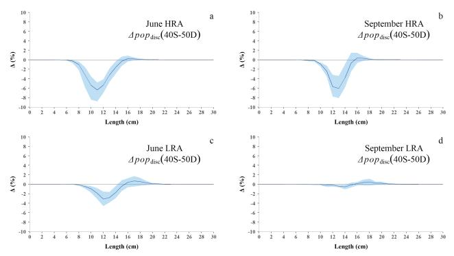
Fig. S2: Difference  $\Delta pop_{disc}(l,a,t,g)$  in the hake discards size structure between 40S and 50D codends in HRA in June (a), HRA in September (b), LRA in June (c) and LRA in September (d). 95% Efron percentile confidence intervales are also given (coloured area around line). 40S: 40 mm square mesh in the trawl codend; 50D: 50 mm diamond mesh in the trawl codend; HRA: high recruitment area, LRA: low recruitment area; ;  $\Delta$  (%): difference in percentage (%).
