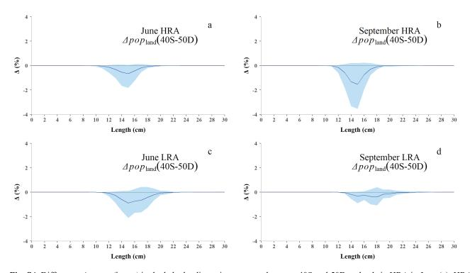
Fig. S4: Difference  $\Delta pop_{land}(l,a,t,g)$  in the hake landings size structure between 40S and 50D codends in HRA in June (a), HRA in September (b), LRA in June (c) and LRA in September (d). 95% Efron percentile confidence intervals are also given (coloured area around line). 40S: 40 mm square mesh in the trawl codend; 50D: 50 mm diamond mesh in the trawl codend; HRA: high recruitment area, LRA: low recruitment area; ;  $\Delta$  (%): difference in percentage (%).
