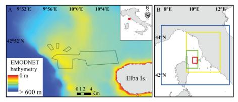
*Fig. 1:* A) Map of the study area with the indication of the area with high resolution bathymetry (black lines); B) North Tyrrhenian grids: regional resolution (1/60) blue, high resolution (1/120) yellow, very high resolution (1/240) green, target resolution area (1/480) red.
