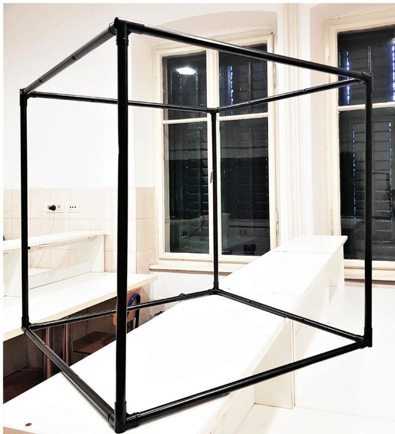
**Figure S1.** A cube frame used for *in situ* observations (dimensions: 0.5x0.5x0.5 m).
