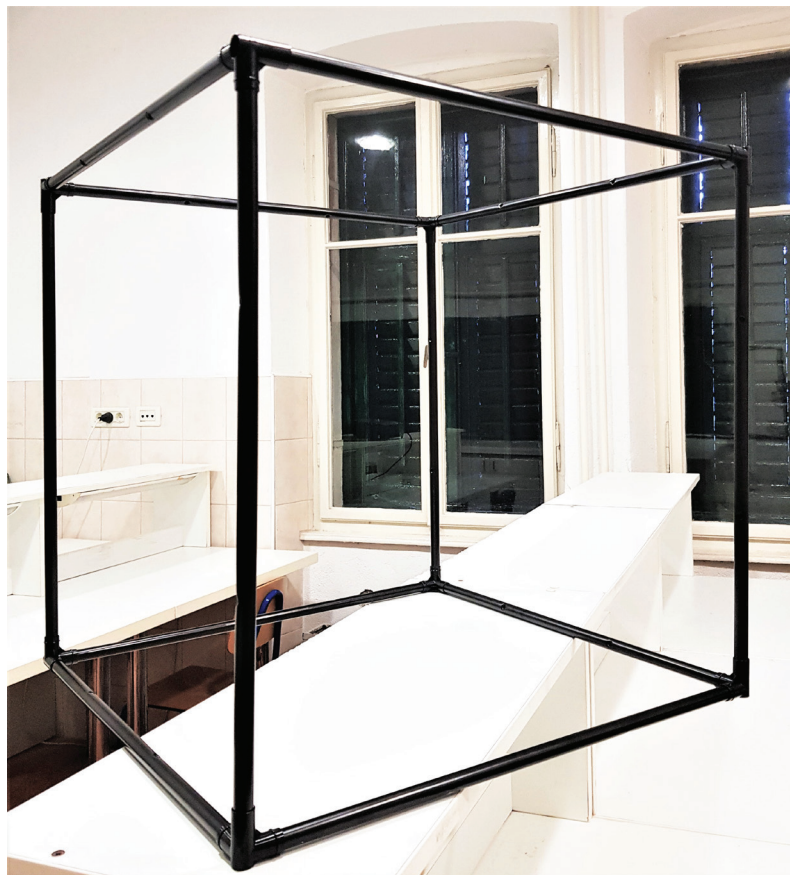
Figure S1. A cube frame used for in situ observations (dimensions: 0.5×0.5×0.5 m).
