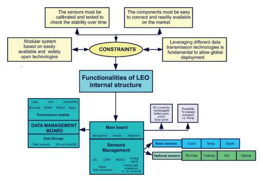
Fig. 2: LEO modularity reflects internal main electronic components distribution and assemblage.
