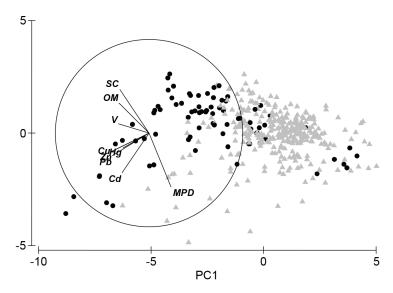
*Fig. 2:* Projection of samples ( $\blacktriangle$ , shallow and  $\bullet$ , deep) on the first plane of PCA based on percentage of silt-clay (SC), mean particle diameter (MPD), organic matter content (OM), and heavy metal concentrations (Zn, Cu, Pb, Cd, V and Hg). Vectors of the linear correlations with individual variables are superimposed on the graph.
