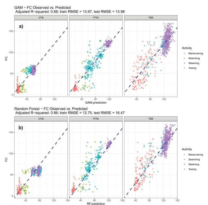
*Fig. 6:* Predictive performance of the (a) GAM model and (b) Random Forest. The image depicts predicted vs. observed values of consumption FC (l/h) for a random sample of 2,000 observations extracted from the test dataset.
