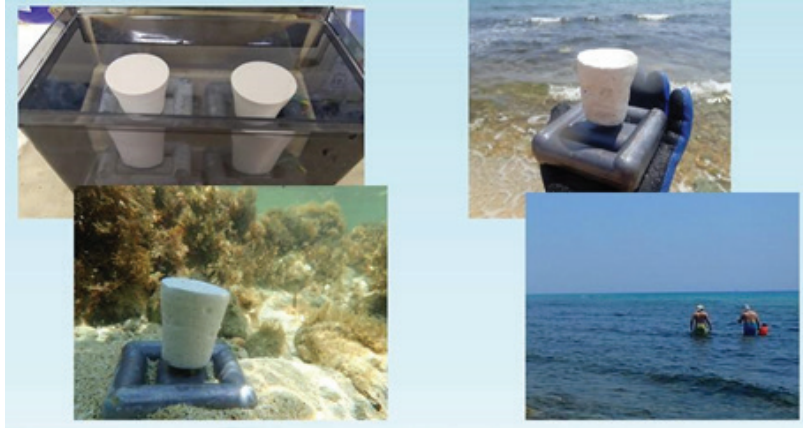
Fig. S3: Placement of gypsum cones in Greek coasts.
