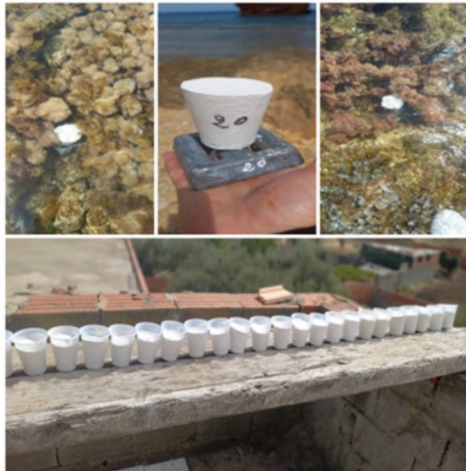
Fig. S4: Placement of gypsum cones in Tunisian coasts.
