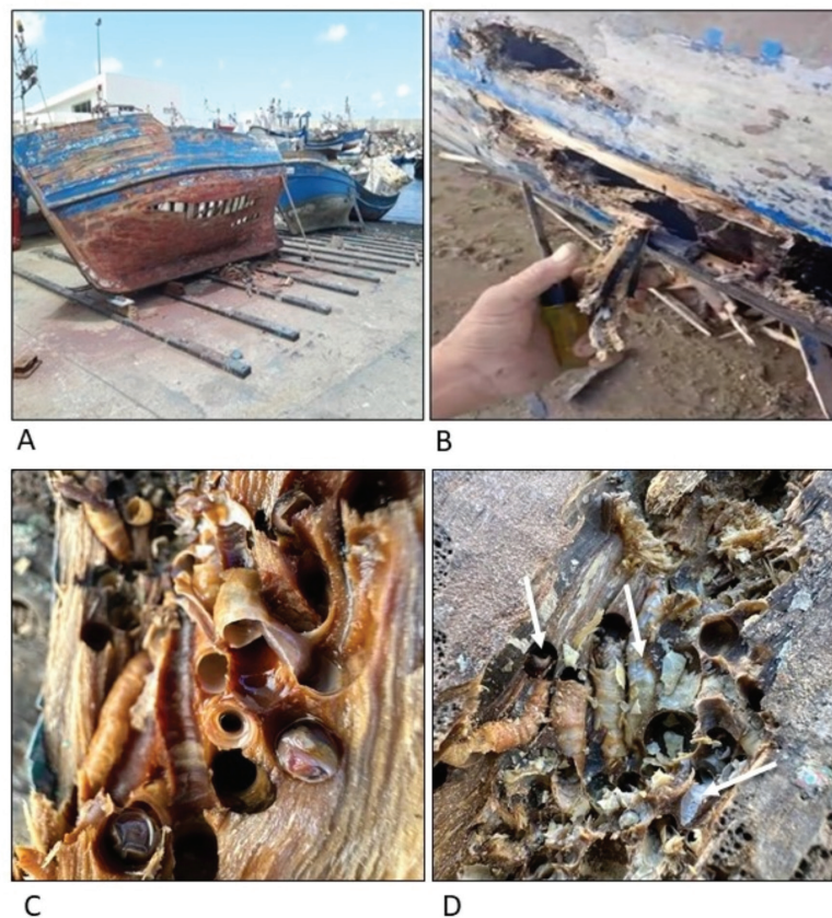
Fig. 2: Teredinid damage to artisanal fishing boats; a- Damaged boats queuing at the shipyard, 2023; b- The magnitude of damage observed on boat hulls; c- Teredinids in a damaged wooden piece from a boat in the new fishing port of Tangier, 2023. d- Shipworm tunnels in the wooden hull of a boat showing the typical calcareous lining (arrows).
