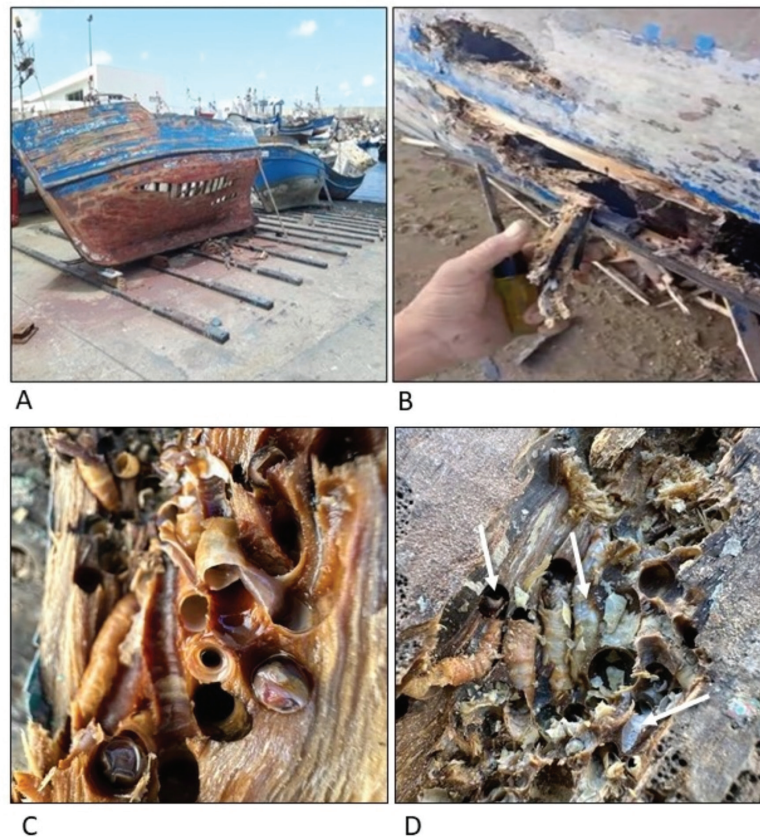
Fig. 2: Teredinid damage to artisanal fishing boats; a- Damaged boats queueing at the shipyard, 2023; b- The magnitude of damage observed on boat hulls; c- Teredinids in a damaged wooden piece from a boat in the new fishing port of Tangier, 2023. d- Shipworm tunnels in the wooden hull of a boat showing the typical calcareous lining (arrows).
